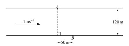
The diagram shows a river which is 120 m wide and is flowing at  $4 \,\mathrm{ms^{-1}}$ . Points A and B are on opposite sides of the river such that B is 50 m downstream from A. A man needs to cross the river from A to B in a boat which can travel at  $5 \,\mathrm{ms^{-1}}$  in still water.
