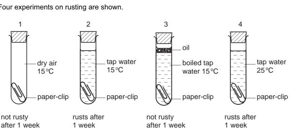
Which two experiments show that air is needed for iron to rust?
