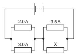
The current in three of the resistors is shown.
