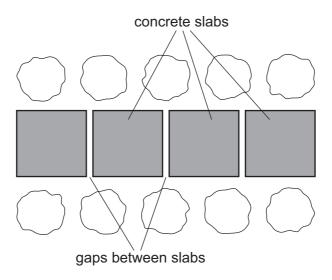
On a hot day how does the size of each slab and the gaps between the slabs change?
