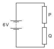
When 2C of charge passes round the circuit, 4J of energy is dissipated in resistor P.
