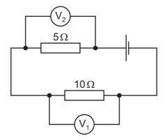
The reading on the voltmeter  $V_1$  is 2 V.
