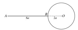
A uniform rod AB, of mass m and length 6a, is rigidly attached at B to a point on the circumference of a uniform circular lamina of mass m, radius 2a and centre O. The lamina and the rod are in the same vertical plane, and ABO is a straight line (see diagram). Show that the moment of inertia of the system about an axis l through A perpendicular to the plane of the lamina is  $78ma^2$ . [4]
