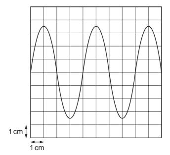
The oscilloscope time-base setting is  $0.5\,\mathrm{ms\,cm^{-1}}$  and the Y-plate sensitivity is  $2\,\mathrm{V\,cm^{-1}}$ .
