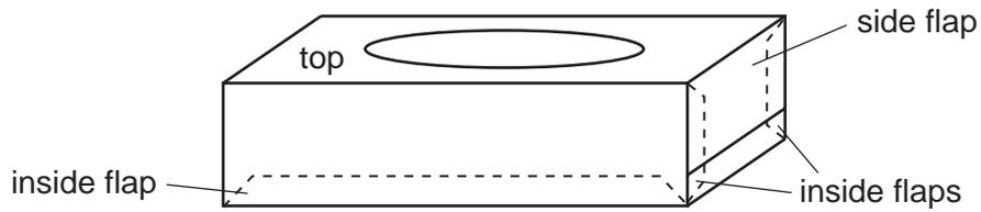
A cardboard container for tissue handkerchiefs as shown above is made up of one piece of cardboard cut and folded to the necessary shape and glued together. The two ends are overlapped and glued and the base is secured to the facing side on the diagram by a glued flap folded from the base. The top has an oval hole which allows the tissues to be withdrawn.
