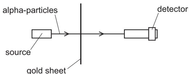
Most alpha-particles pass straight through the thin gold sheet.
