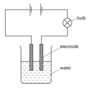
After the student adds substance  $\mathbf{X}$  to the water, the bulb lights.
