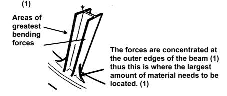
(ii) Joists in a building structure. [1]
