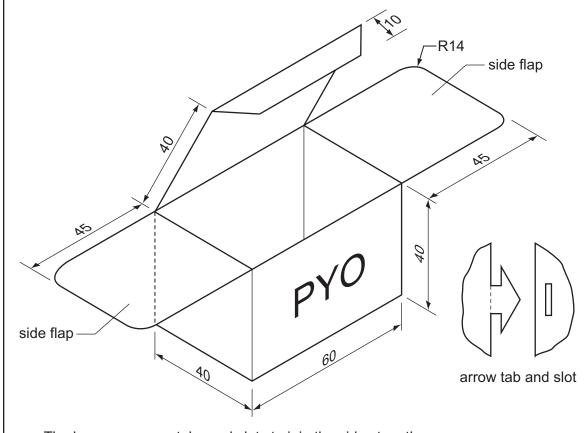
The box uses arrow tabs and slots to join the sides together.
