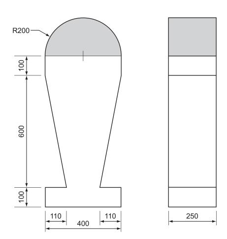
In the space to the right, draw an isometric view of the ice-cream model to a scale of 1:5. [10]
