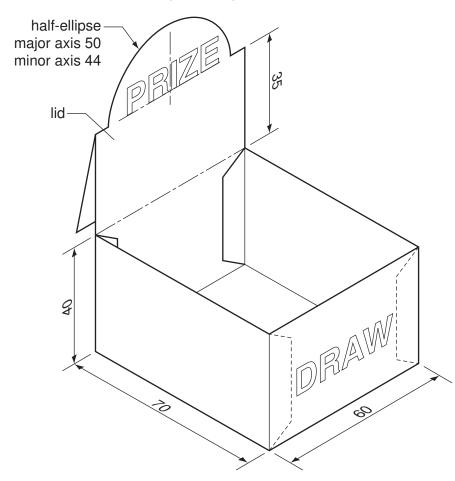
(a) In the space on the right, complete the drawing of a full-size, one-piece development (net) of the box. The front of the box and one glue tab have been started for you. Include the remaining glue tabs required to make the
