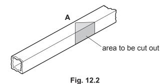
Use sketches and notes to show how the joint could be cut out and the edges made flat using hand tools.
