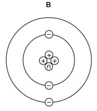
key  $\bigcirc$  = a neutron + = a proton  $\bigcirc$  = an electron (not to scale)
