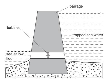
At low tide the water is allowed to flow back into the sea through a turbine.
