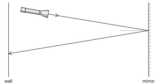
incident ray in line with axis of torch, reflected off mirror, hitting wall; angle of incidence and angle of reflection reasonably equal on visual inspection;
