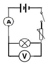
voltmeter correctly connected in parallel with lamp only; other components all in series; [accept equivalent circuits, variable resistor in any position other than in parallel with voltmeter]
