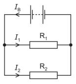
The current in the battery is  $I_{B}$ . The current in  $R_{1}$  is  $I_{1}$  and the current in  $R_{2}$  is  $I_{2}$ .
