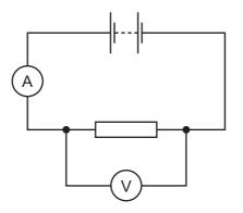
The reading on the ammeter is 2.0 A and the reading on the voltmeter is 4.0 V.
