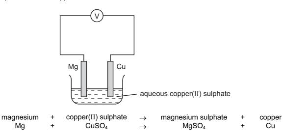
It can be deduced that magnesium is ....1... reactive than copper and that the mass of the deposited copper is ....2.... the mass of the dissolved magnesium.
