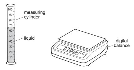
The student records the volume of the liquid from the scale on the measuring cylinder. He then puts the measuring cylinder containing the liquid on a balance and records the mass.
