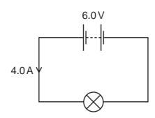
A current of 4.0 A flows in the circuit for 20 s.
