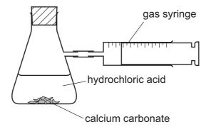
The time to collect 50 cm<sup>3</sup> of gas is measured.
