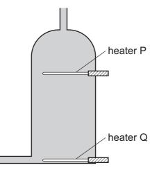
When only heater Q is switched on, it takes a long time to heat the tank of water to 60 °C.
