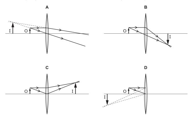
34 Which ray diagram represents the formation of a virtual image I of an object O?
